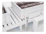
suppression with **Power PinPoint LED** for detecting small objects, for precise edge detection and for detecting shiny, color-textured objects
