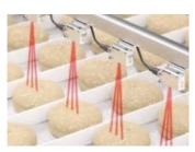
Dynamic reference diffuse sensors (DRT) for **objectindependent detection** with the conveyor belt as a reference.
